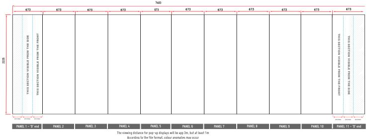
We print with a tolerance of 0.1 to 0.2% so a difference of 1mm up to 5mm is normal within a height of 230cm
